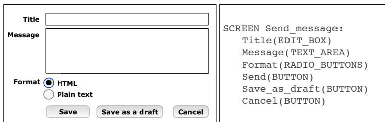
Fig. 1. A simple screen and its corresponding specification in ScreenSpec
