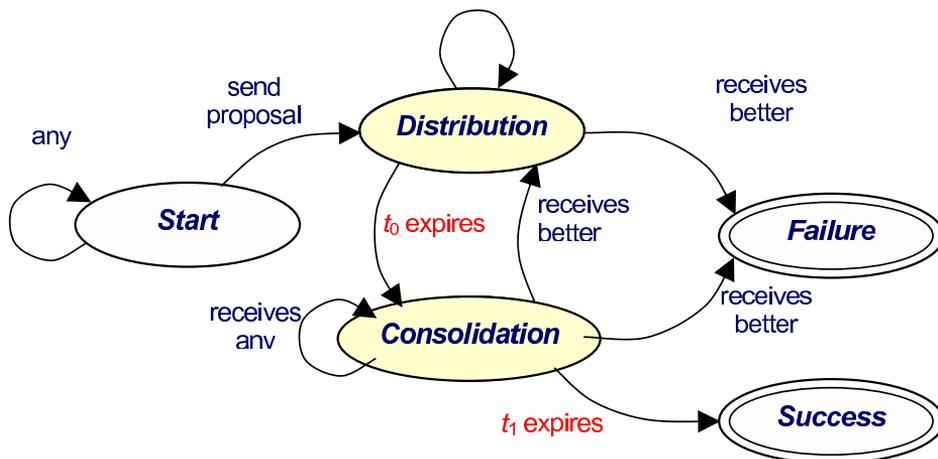
Fig. 1. State diagram of the coordination protocol
