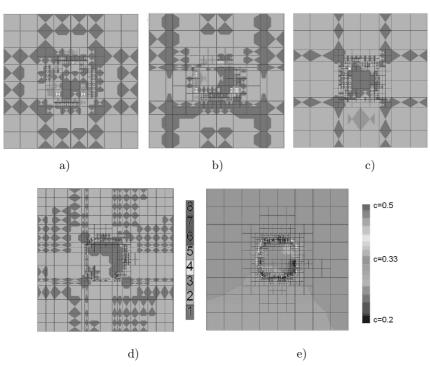
Fig. 4. Four optimal meshes obtained after 10 iterations from the first, second, third or fourth initial mesh, respectively. Different colors denote different polynomial orders of approximation on finite element edges and interiors. The last panel presents resulting concentration field distribution computed on one of the optimal meshes
