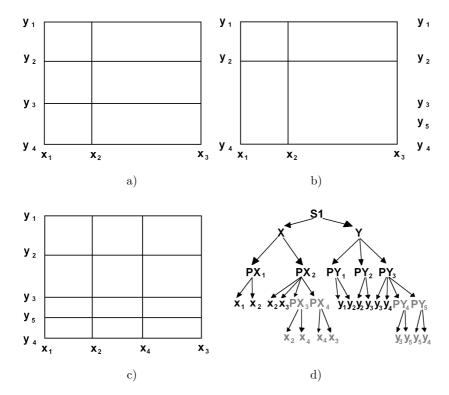
Fig. 6. a) phenotype before mutation, b) phenotype after mutation – removing of the component, c) phenotype after mutation – splitting of the component, d) hierarchical chromosomes corresponding to the mesh from panel c)
