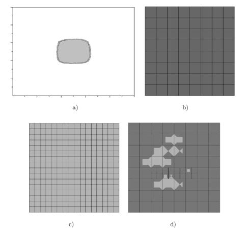
Fig. 1. a) Exemplary fraction of the solid phase obtained by CA simulation described in [7]; b) c) d) Coarse, fine and optimal meshes for the first iteration. Different colors denote different polynomial orders of approximation on element edges and interiors
