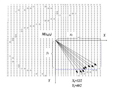
Fig. 2. The point M is the center of the image with the coordinates  $X_k = 32/2$  and  $Y_k = 40/2$  (total number of pixels on the x and y axes divided by 2, respectively)
