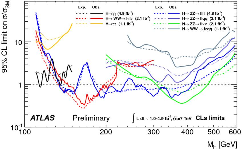
Figure 1. The expected (dashed) and observed (solid) cross-section limits for the individual search channels, normalized to the Standard Model Higgs boson cross section, as functions of the Higgs boson mass. These results use the profile likelihood technique with 95% C.L. limits using the  $CL_s$  prescription.
