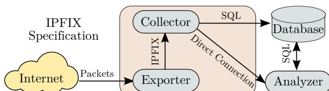
Figure 2. General architecture of a monitoring platform implementing IPFIX
