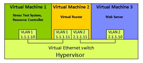
Figure 4. High-level logical depiction of the experimental cloud server and network testbed
