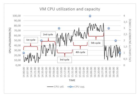
Figure 6. Virtual router VM CPU utilization and capacity over time
