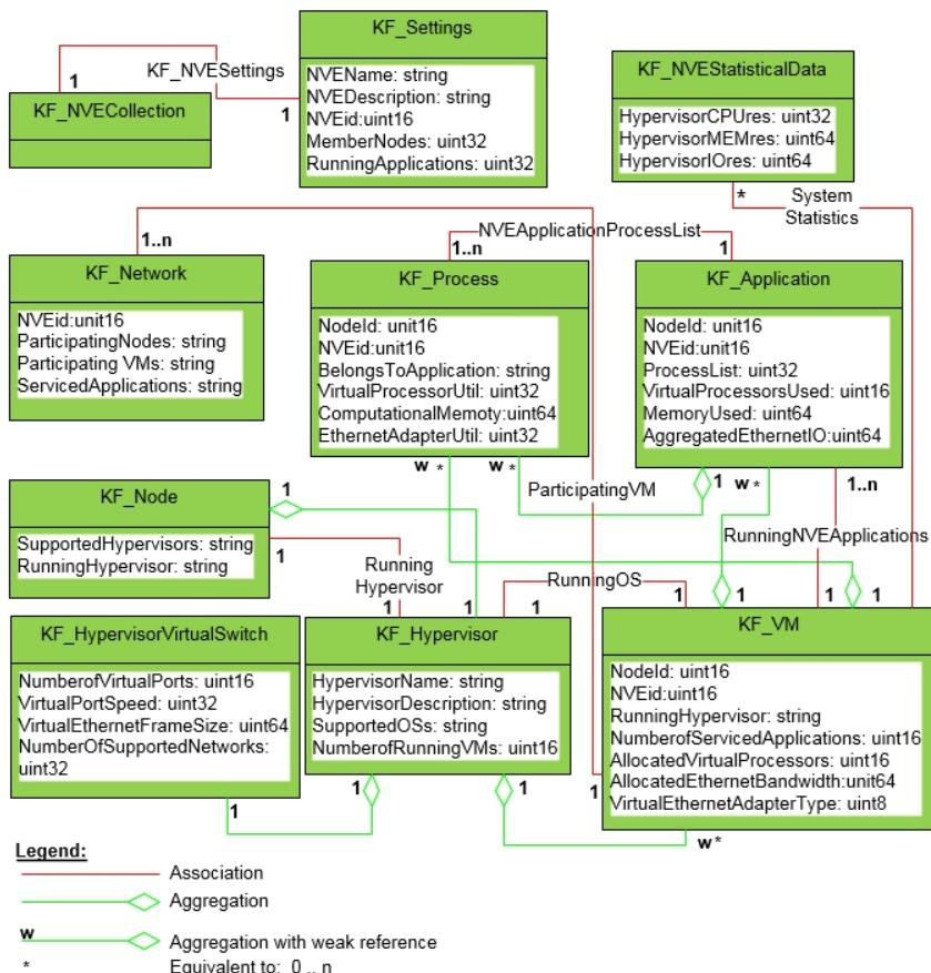
Figure 3. UML diagram of model classes, their properties and associations
