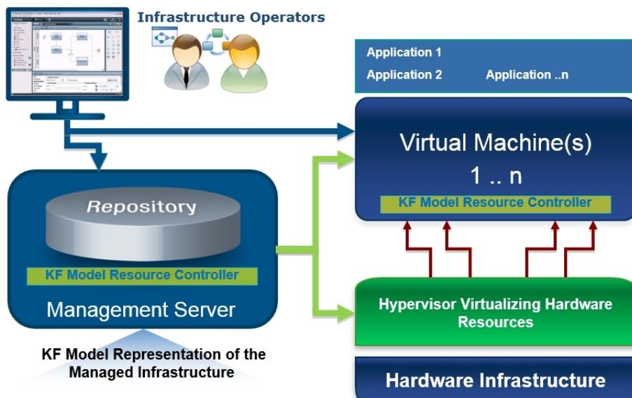
Figure 2. Management environment architecture using the proposed model
