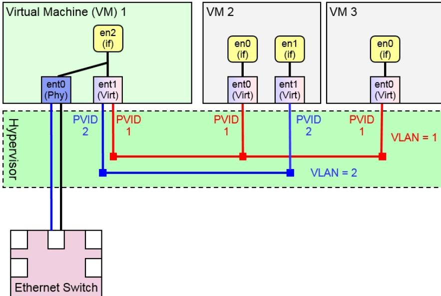
Figure 1. High-level architecture of systems networking based on the hypervisor IEEE 802.1Q virtual switch
