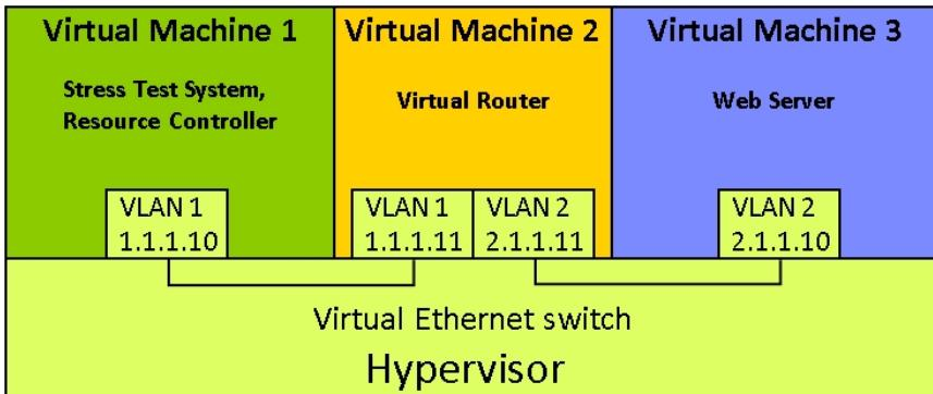
Figure 4. High-level logical depiction of the experimental cloud server and network testbed
