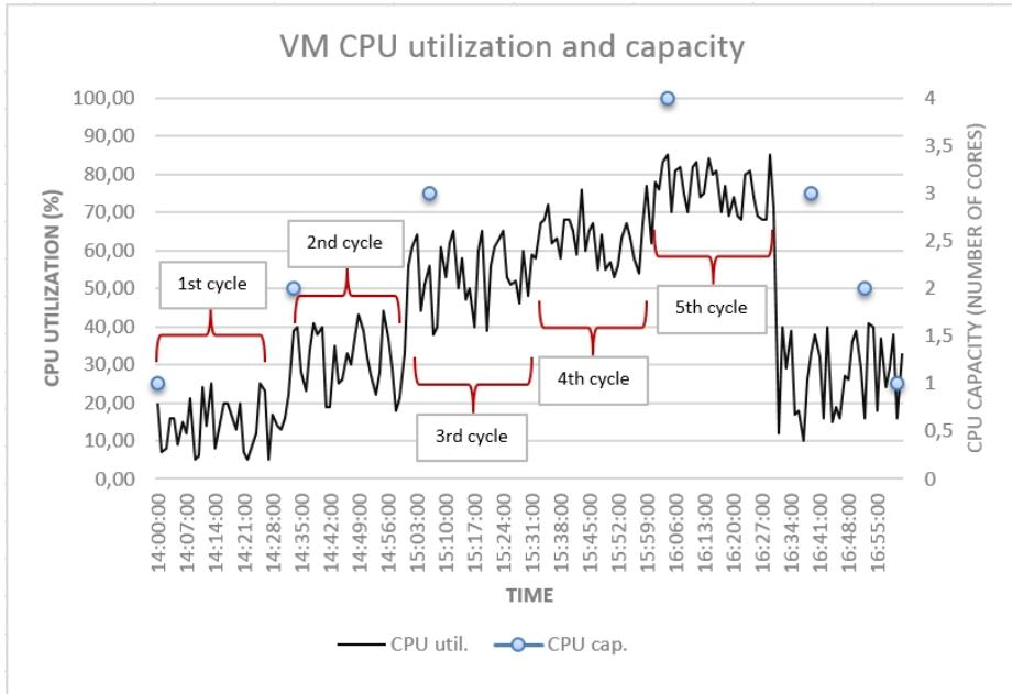
Figure 6. Virtual router VM CPU utilization and capacity over time
