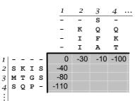
Fig. 3. A detail of the dynamic programming matrix for profile alignment
