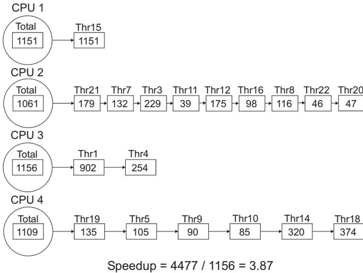
Fig. 3. Load distribution obtained with the CYCLIC algorithm
