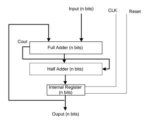
Fig. 12. Modulo  $2^n - 1$  adder architecture
