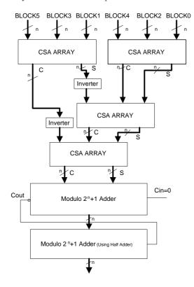
Fig. 7. Architecture for converting to diminished-1 for 6 blocks
