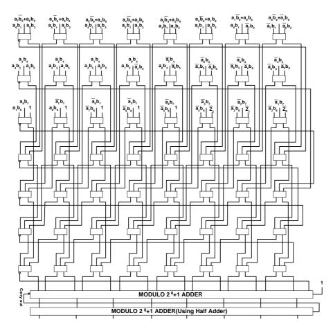
Fig. 5.  $2^8 + 1$  modular multiplication architecture
