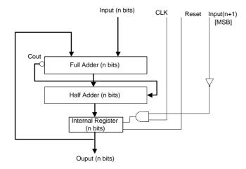
Fig. 11. Modulo  $2^n+1$  adder architecture
