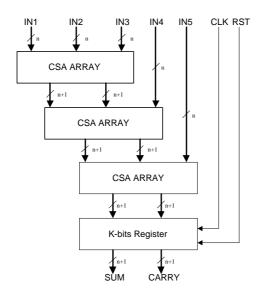
Fig. 1. Block diagram of five-to-two CSA
