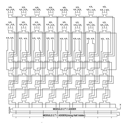
Fig. 8.  $2^8-1$  modular multiplication architecture
