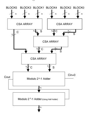
Fig. 10. Architecture for converting to modulo  $2^n - 1$  for 6 blocks
