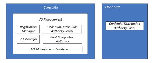
Figure 4. Structure of the XtreemOS VO management service
