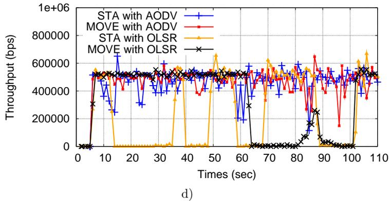
Fig. 6. Throughput results of simulation: a) Source node #1 → destination node #2, b) Source node #1 → destination node #3, c) Source node #1 → destination node #4, d) Source node #1 → destination node #5
