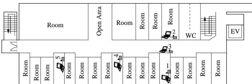
Fig. 1. STA model (using iptables). Node #1 is accessible via node #3. When the destination node is #2, the hop distance is 2, i.e.  $1 \rightarrow 3 \rightarrow 2$ .
