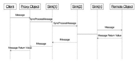
the chain of client and server sinks to the remote object.
